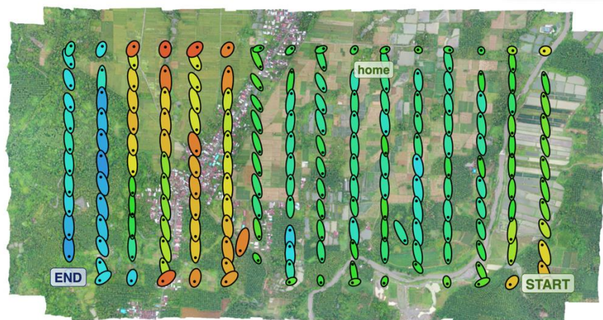
Figure 1. Flight plan for aerial imagery acquisition
