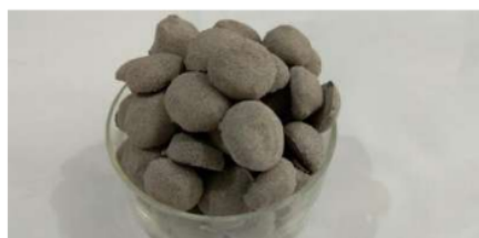
Figure 1. Pellet of CSiMN Composite
