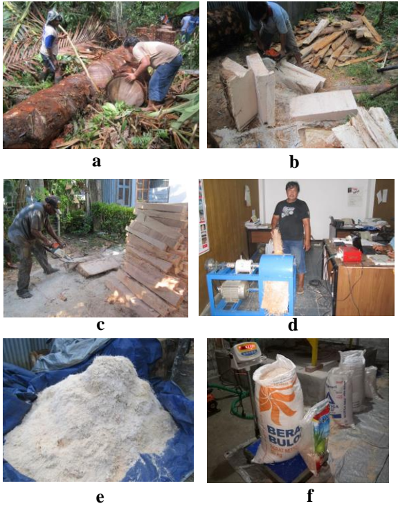
(a) Ready harvested sago trunk was felled down, then cut into logs, (b) Debarking and splitting the log (c) Pieces of sago log called batten was ready to be rasped, (d) Sago log pieces is being rasped, (e) Rasped sago log/sago pith called repos , (f) Weighing the rasped pith.
