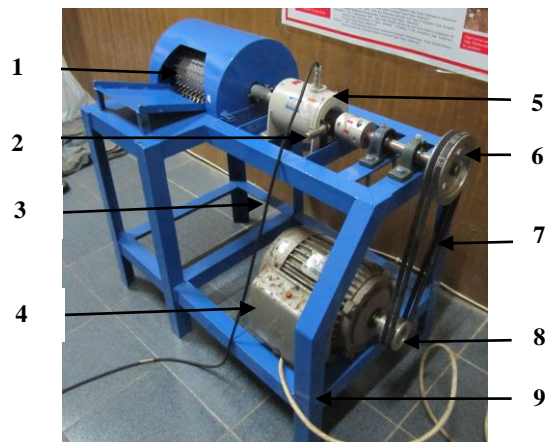
Note: (1) Cylinder, (2) Tachometer sensor, (3) Connecting cable to the torque sensor interface, (4) Electric motor, (5) Torque meter, (6) Driven pulley, (7) V-belt, (8) Driver pulley, (9) Main frame.
