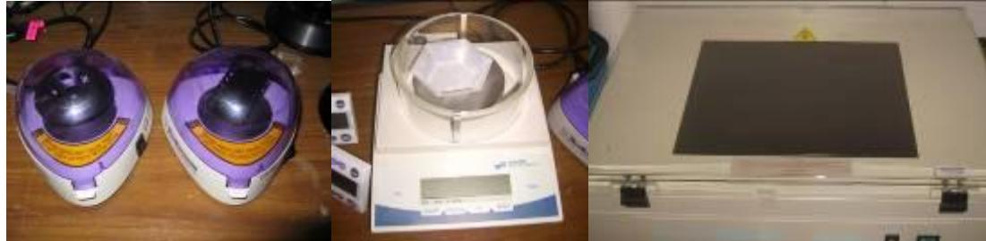
Mikrosentrifuge Timbangan UV Transluminator
